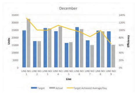
In the chart above, it is seen that line No 6 has improved to achieve the target by December but line No 7 and 9 could not meet the target provided and proceeded with low efficiency to the negative side. In December, line 7 and 9 working efficiency decreased more than in November. Therefore, we narrowed our analysis to focus on line 7 and 9.
